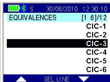
Select the desired CIC or EIC code (depending on the *Show EIC/CIC* setting), and then confirm by pressing SEL. LINE in order to see the equivalence (see image below).
