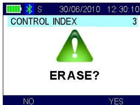
If the *Erase* function is confirmed, the device removes the selected data-set from the current control-file.
