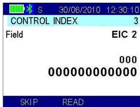
In the case the field repetition number is greater than needed, press SKIP to finish the field.
