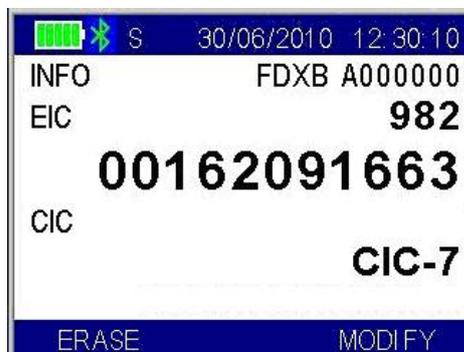
In both searching modes, to delete the data-set, press ERASE, the device asks for confirmation (YES or NO).
