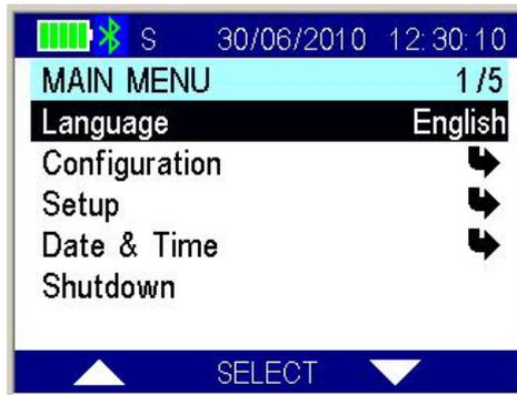
You can scroll through the menu by pressing the UP or DOWN which are the contextual keys on the right and on the left of the ON button. The arrows located on the right of the display means that this menu contains a sub menu. In order to enter a sub menu, you have to press the ON button while it is highlighted.
