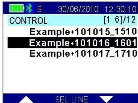
Move through the list using the UP/DOWN buttons and press SEL.LINE to choose the desired file.
